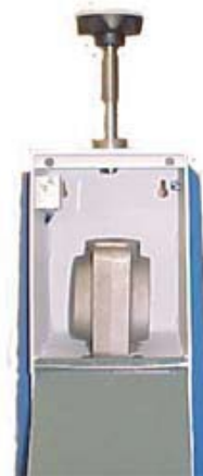
(Fig. 2) The screw handle must be completely up when removing the flask
