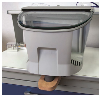
Coupling to a peg with suction (Jeb type).
