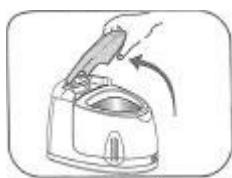
7. When the cleaning is finished, unplug the unit and open the lid to remove the basket and the item.
