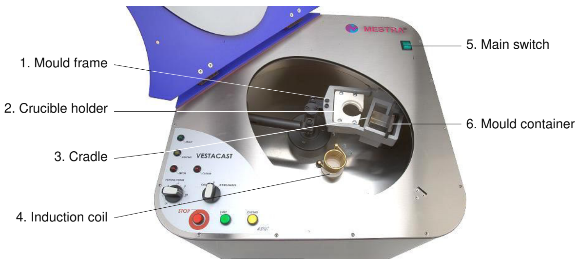
Fig. 2: Casting chamber with centrifugal arm
